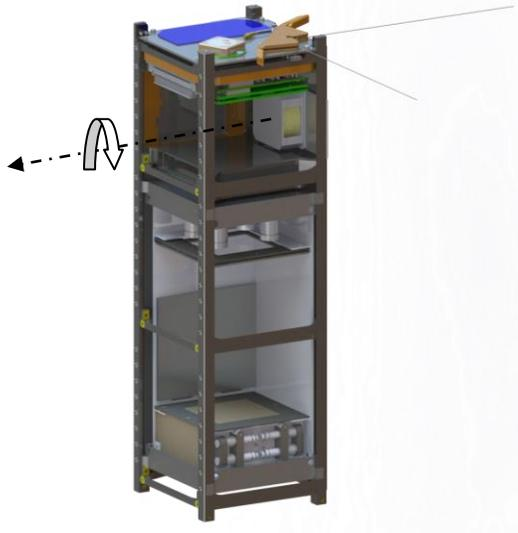
**Figure 2. AOSAT-1 Model with its spin axis.**
